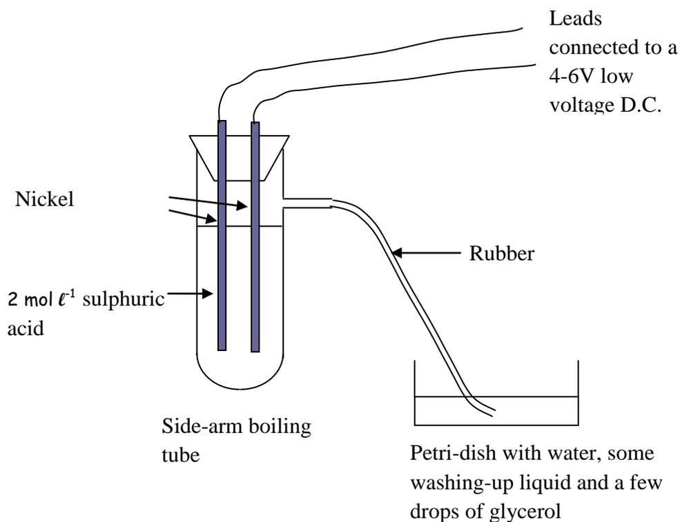
2. Turn on the electricity and allow the gases produced to escape for a few minutes. This flushes any air out of the apparatus as this will reduce the effect on igniting the gases.
