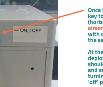
Once installed switch the key to the 'on' position (horizontal) and email airsensor@sepa.org.uk with confirmation that the sensor is active.
