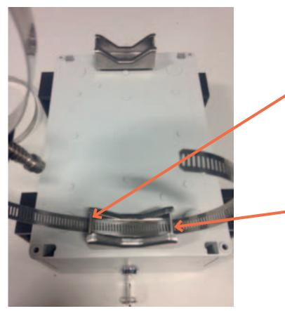
Thread the end of one of the adjustable straps through the bottom holder. Then take the second adjustable strap and thread it through the top holder.
