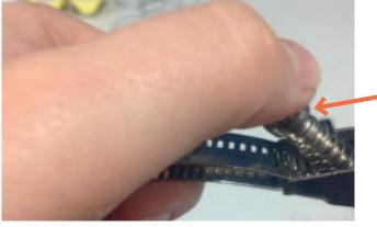
Push the screw fastenings down to secure the straps. Tighten the fastenings with a screw driver to ensure the sensor is fully secured.
